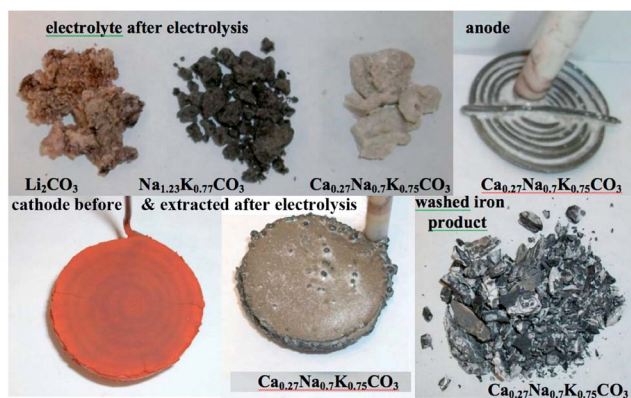
Fig. 2 Left: the iron molten air battery starting with an (uncharged) pressed Fe 2 O 3 pellet cathode bottom left photo in several molten carbonate electrolytes. Fe 2 O 3 is soluble in Li 2 CO 3 (as LiFeO 2 , with addition of Li 2 O), but not in sodium or potassium carbonates. A variety of carbonates can promote iron electrodeposition, without Fe(III) lithiation dissolution, such as the Ca 0.27 Na 0.7 K 0.73 CO 3 (shown). 17 Bottom: two photographs of the battery cell configuration.
