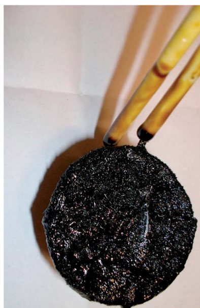
Fig. 14 The \text{VB}_2 molten air battery. Photo: \text{VB}_2 formed on the steel wire cathode, extracted following an 8.5 hour charge at 0.2 A in a \text{Li}_2\text{O}-\text{V}_2\text{O}_5-\text{B}_2\text{O}_3 electrolyte. FTIR analysis of this electrode is described in the text. Right: 100 ohm discharge potential subsequent to a 0.2 A charging for 10 minute, in 2 g of various 800 °C vanadate borate electrolytes sandwiched between a coiled disc nickel ( 4 \text{ cm}^2 area coiled 1.0 mm diameter wire) electrode above and a coiled disc steel ( 3 \text{ cm}^2 area coiled 1.2 mm diameter wire) electrode.
